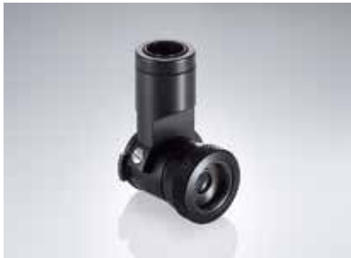
GOA2, Autocollimation eyepiece To perform autocollimation with any TPS instrument except TS02+. The 394787 GEB62 plug-in lamp and 394792 GEB63 battery box are additionally required. Order No: 199899
